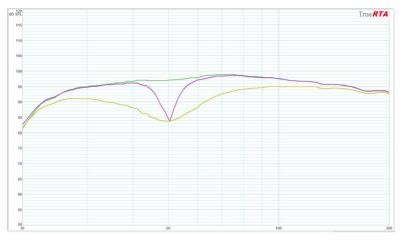
**Measuring The In-Room Frequency Response:** In order to use the PEQ effectively, you must measure the in-room FR of the subwoofer at the listening positions. This can be done manually using test tones and an spreadsheet, or it can be accomplished using software such as "TrueRTA", or "Room EQ Wizard". SVS does not provide technical support on the setup and use of any software, but it can make measuring the subwoofer FR easier and faster than manual methods.
